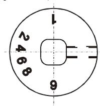
position **9 = soft** (clockwise direction) position **1 = firm** (counter- clockwise direction)
