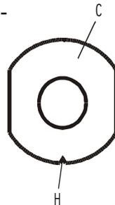
Orient the score mark (H) on adjusting head in the center of any of the four sides of the square rod stop. Then lock the parts together by screwing the lock nut up to the adjuster head.
