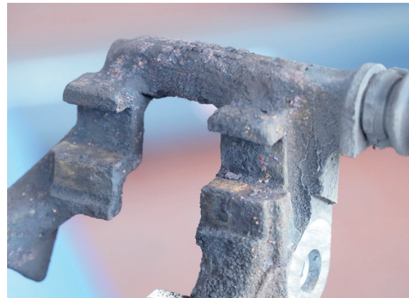
Corroded pad guidance
