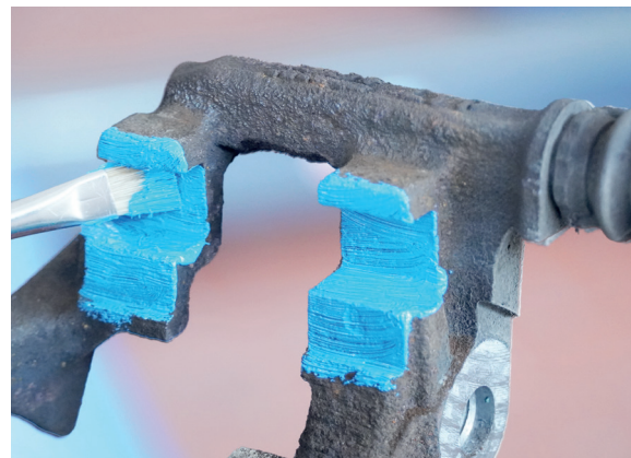
Pad guiding treated with NOxidation
