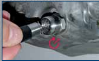
2. Connect drain tube and turn a quarter turn to lock into place.
