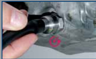
4. Disconnect drain tube with quarter turn and remove.
