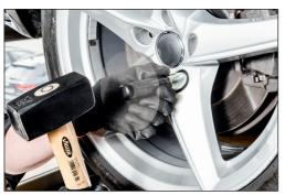
Drive this unit into the rim lock, so that the malleable rim lock can work its way into the profile.
