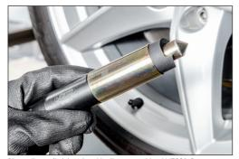
Place the suitable wheel bolt removal tool V7001-3 or V7001-4 in the V7001-1 tool holder. Make sure that it is securely gripped and locked in the lock washer.
