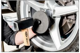
Once the malleable rim lock has been snugly driven into the rim lock, the rim lock can be removed by hand using a ratchet.
