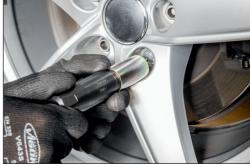
Place the tool holder with suitable malleable rim lock and rim protection on the rim lock.
