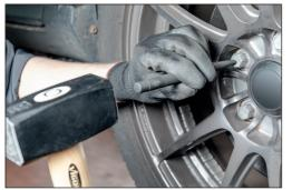
Use the centre punch to strike the contact surface into the wheel bolt as a guide.
