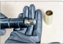
Place the suitable malleable rim lock in the V7001-1 tool holder. Make sure that it is securely gripped and locked in the lock washer.
