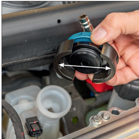
Fig. 4 Spread the arms of the adapter.
