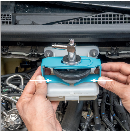
9 pav. Suspauskite laikiklius.
