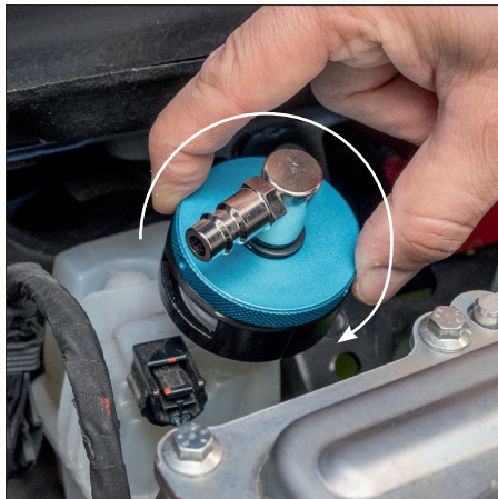
Fig. 6 Close the arms and turn the top cover to secure the adapter.
