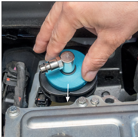
Fig. 5 Press the adapter down into the brake fluid reservoir.
