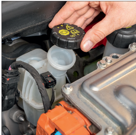
Fig. 3 Remove the cover of the brake fluid reservoir.
