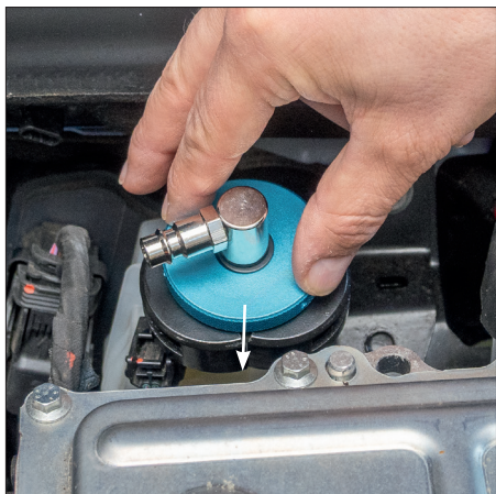
Joon. 5 Vajutage adapter alla pidurivedeliku mahutisse.
