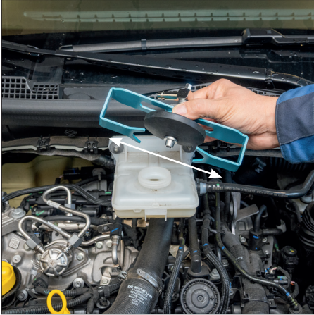
Fig. 7 Open the arms of the universal adapter.
