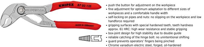
KNIPEX Cobra® - the Hightech Water Pump Pliers. No more time-consuming presetting of the required opening size. Just position the upper jaw to the workpiece, push button and move close the lower jaw, ingeniously simple.
