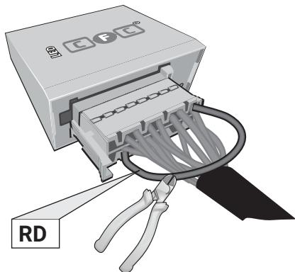
**Pin 11 and Pin 2 disconnected**
