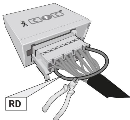
Pin 11 and Pin 2 disconnected
