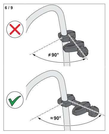
► Align the spacer with the mounting bracket.
