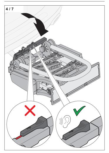
► Push the clamping lever with a force that complies with a weight of 35–45 kg down until it engages.
