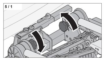
▶ Loosen the two star knobs for the mounting bracket.
