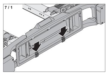
▶ Ensure that the registration clamps are pushed down.
