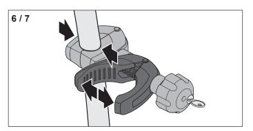
► Attach the bracket clamp to the bracket by opening or pulling apart and spreading the bicycle clamp.
