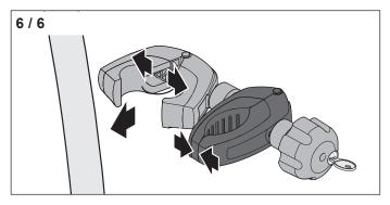
▶ Press the bicycle clamp together to be able to open the bracket clamp.
