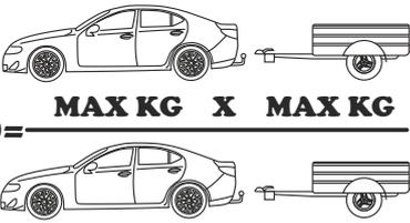
$$D = \frac{\text{MAX KG} \times \text{MAX KG}}{\text{MAX KG} + \text{MAX KG}} \times 0,00981 \leq 8,96 \text{ kN}$$
