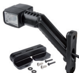
Marker Light Left ADR/GGVS Checked Super Seal 12 - 24 V
