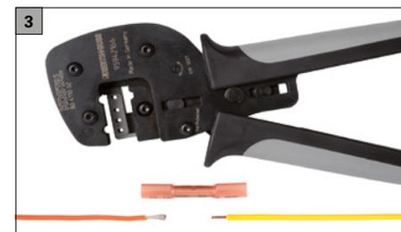
A crimp or shrink connector for example can be used for connection. These connectors are included in the scope of delivery.
