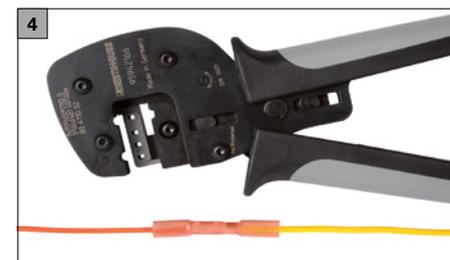
The cables are then crimped with the connector one after the other. In this example with our crimping pliers CrimPro30, alternatively with CrimPro10.
