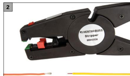
The repair line merely has to be connected with the cable in the vehicle (shown here in yellow). Both cables must be stripped beforehand (e.g. with our stripper).
