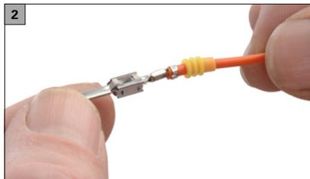
Slide the ELA onto the end of the wire while offset by 180°.
