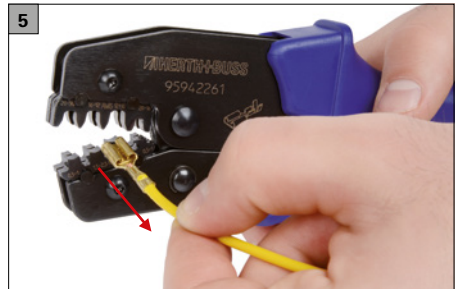
5 Remove the crimped terminal.
