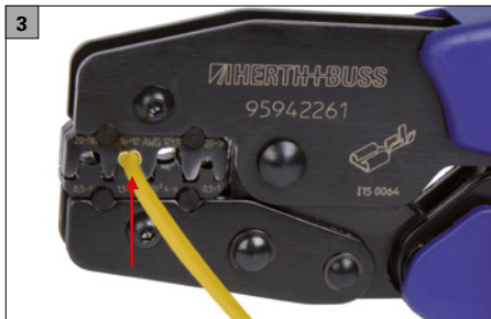
3 Insert the correct stripped wire into the terminal.
