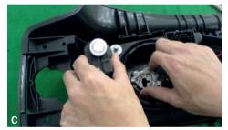
Hold the reflector and install the original motor.
