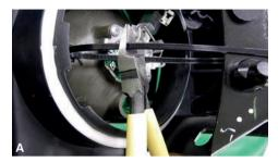
Cut the cable tie with the tool. Remove the cable tie.
