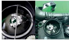
Open the socket securing spring and take down the iron brace.
