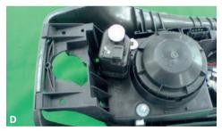
Install the bulb in the relevant specification and cover with the protective cover.
