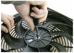
Tighten nut again (Torque: 15 Nm) Remove contact plug carefully
